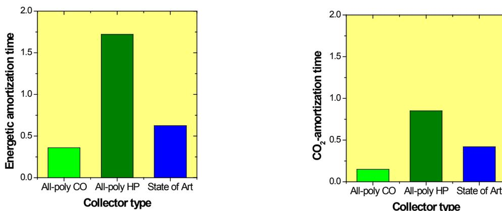
Source: Kicker (2009). All-poly CO = all-polymeric collector made of commodity plastics, All-poly HP = all-polymeric collector made of high performance plastics, state of art = state of the art collector.
