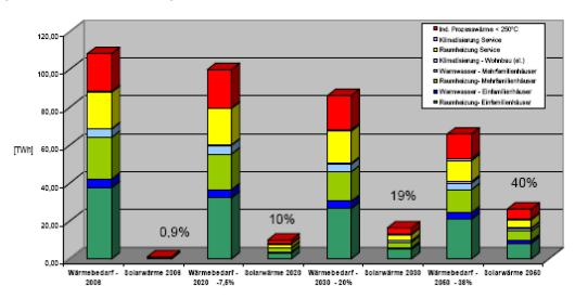
Figure 10.7: Short and long-term potential of solar heat in Austria
