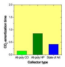
Source: Kicker (2009). All-poly CO = all-polymeric collector made of commodity plastics, All-poly HP = all-polymeric collector made of high performance plastics, state of art = state of the art collector.
